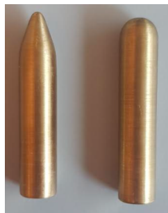
Figure 8: The tips used in the measurements on the balloon. The sharp tip on the left and the dull one on the right.
