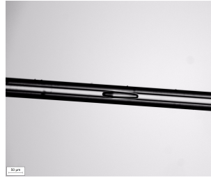
(b) An air bubble in the fiber's core, 20x.
