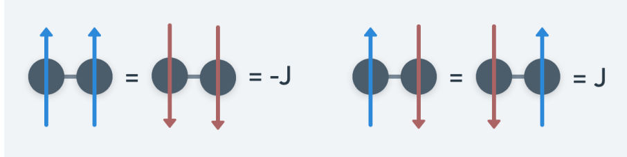
Figure 3: An upward spin has the value 1, while a downward spin has the value -1. The product of two spins in the same direction multiplied by a negative constant will always yield a negative energy contribution. The product of two opposite spins multiplied by a negative constant will instead yield a positive energy contribution.
