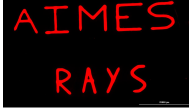
Figure 10: Fluorescent microscopy of printed letters AIMES and RAYS with rhodamine supplement (appearing in red). G-code was developed manually (see Appendix for complete G-code). Printed with nozzle diameter of 410 \mu m. Scale bar = 10000 \mu m.
